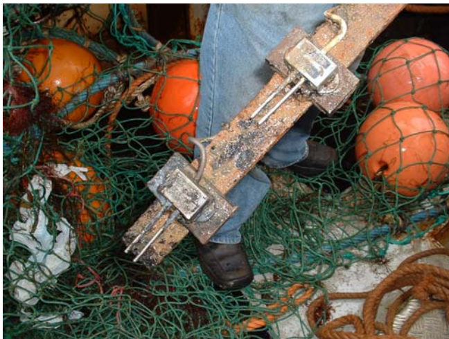
Two Cruz Pro sensors after five months in the bilge of the fishing vessel, Carousel.
